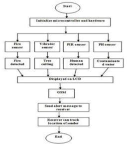
Fig.7. Data flow diagram of forest monitoring system
