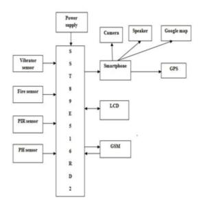
Fig.1. Block diagram of forest monitoring module
