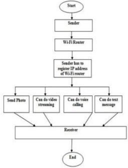
Fig.8. Data flow diagram of communication between sender and receiver via Wi-Fi router
